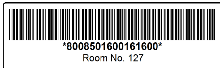
Fig 3. 16-digit Code which Coded using Code-39 form
