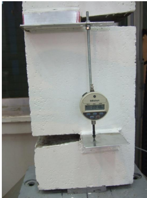
Fig. 2: Measurement of slip across shear-transfer plane
