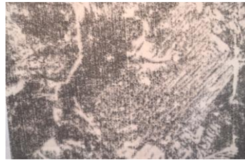
Fig. 2, Ferrite at prior austenite grain boundaries, acicular structure is probably bainite, pearlite matrix (dark area)
