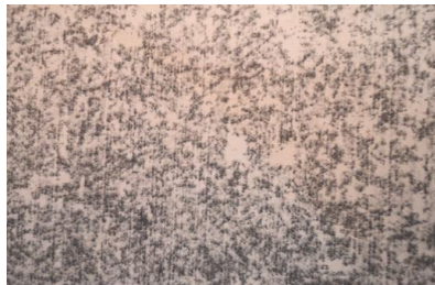
Fig. 11, The specimen 2 same structure in tempering at 460°C showed tempered martensite in uniform condition.
