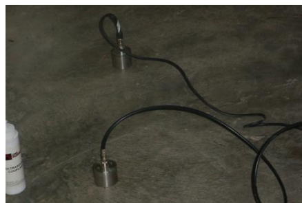
Fig 4: Distance between transmitter and receiver on concrete slab
