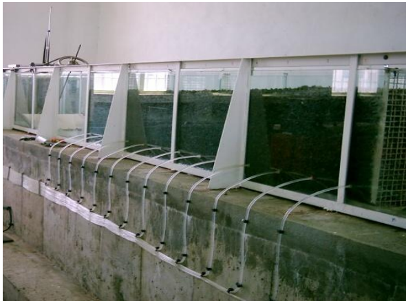
Fig.2: Situation of piezometers from each other
